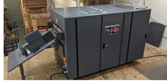
UV coater, puts a protective and attractive coating on the book cover
