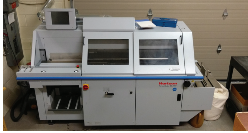
Book binding machine, attaches the cover to the spine
